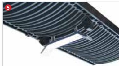
5 Fix the M6 security screws and clamp the grating as shown.
