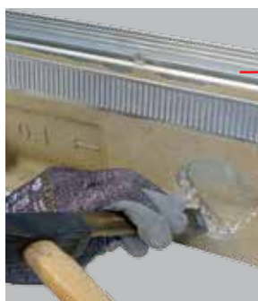
knocking out the recess
