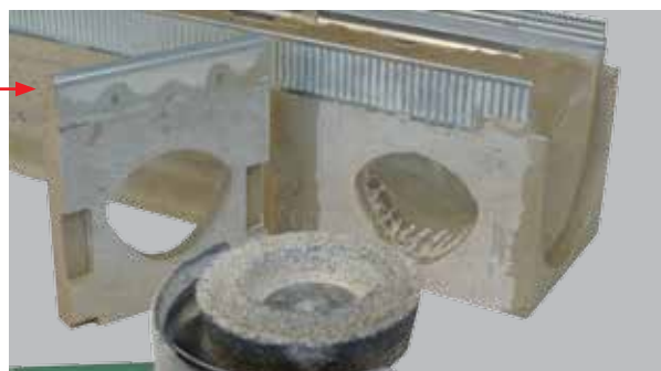
grinding the adhesive surfaces
